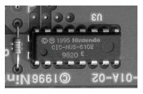
Each cartridge contains a small microcontroller (CIC) that maintains constant communication with a similar chip (PIF) inside the N64 console. If the chip is absent, the wrong type, or does not exactly match the region, the system will not boot.
